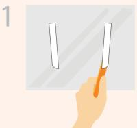
Slide the end of the removal tool under the rails, starting at the bottom.
