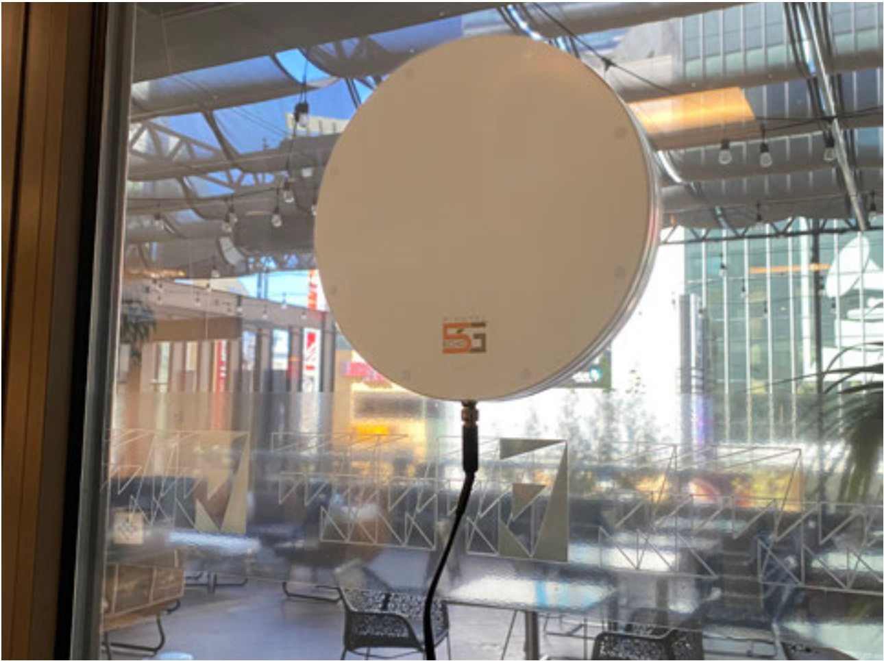
Fig 5 | Inside glass-attached Echo floods Figueroa Room with mmWave.
