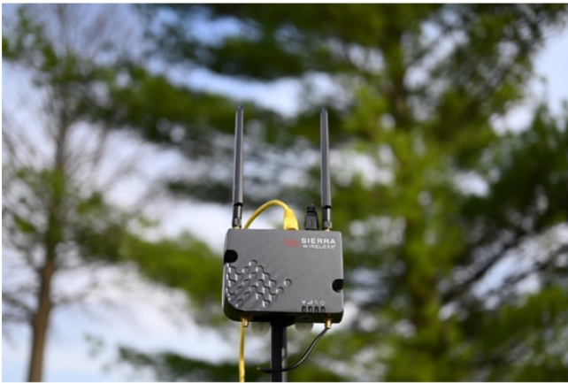
Figure 3: Sierra CPE with omnidirectional antenna
