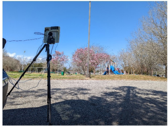
Figure 4: Sierra CPE connected to HBF antenna
