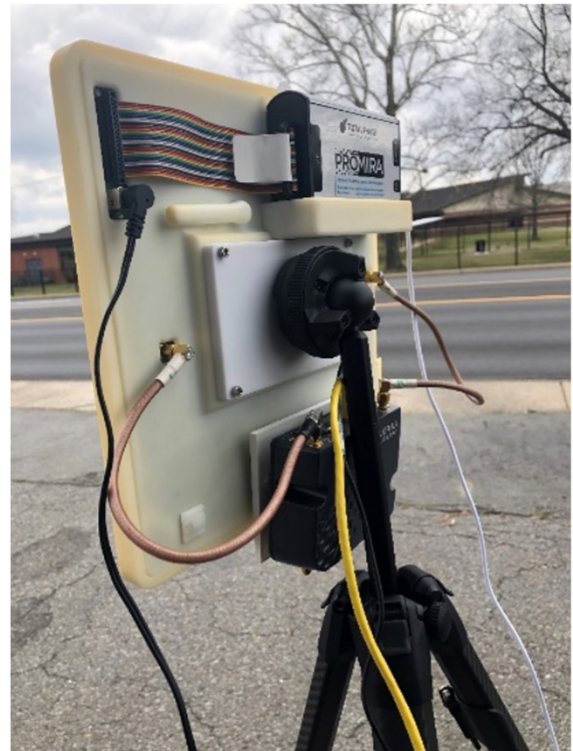
Figure 5: Close up of HBF antenna connected to Sierra CPE
